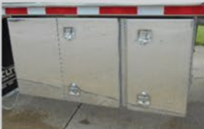
60" Wide Three Door Cabinet to House Overfill System and Controls
